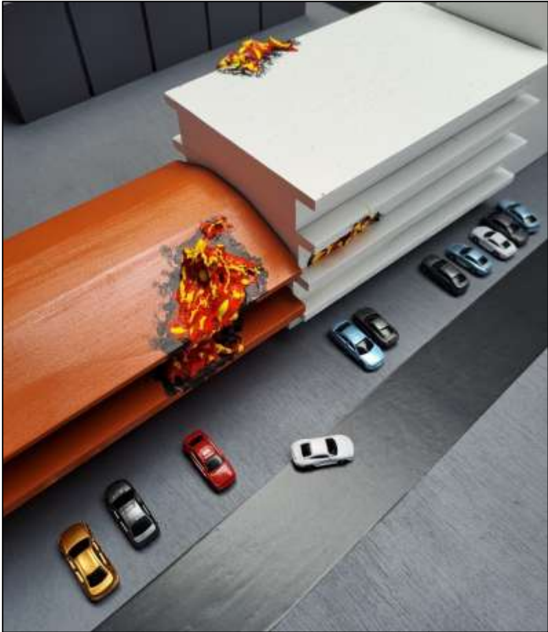
The fire spread from the hotel to the adjacent apartment block has fire established on both sides and different levels of the apartment block.
